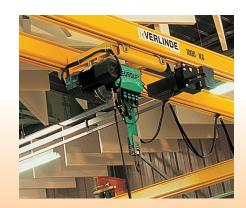
These hoists feature a travelling trolley (for horizontal movement of the load). They are capable of lifting a load of up to 2,000 kg and moving it horizontally in a straight or curved EUROSYSTEM profile.
